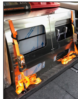
1.3.4 Straps holding back of kitchen to floor
